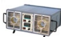
MICRO OIL BATH Model: MOB: 250 Range: 50 to 250°C
