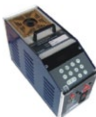
HIGH TEMPERATURE Model: 1200 HN Range: 300 to 1200°C
